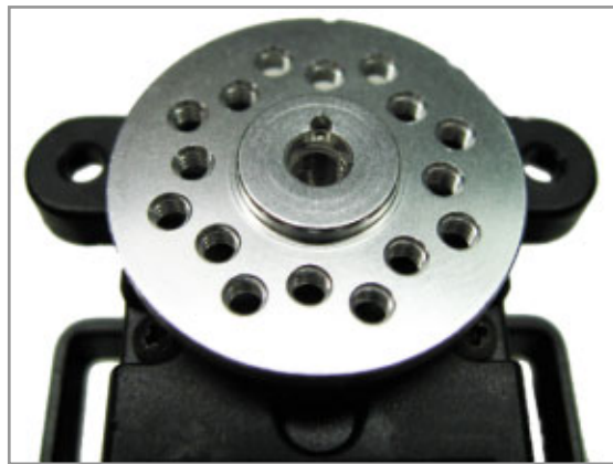
Fig. 2.4 Assembles at Neutral position
